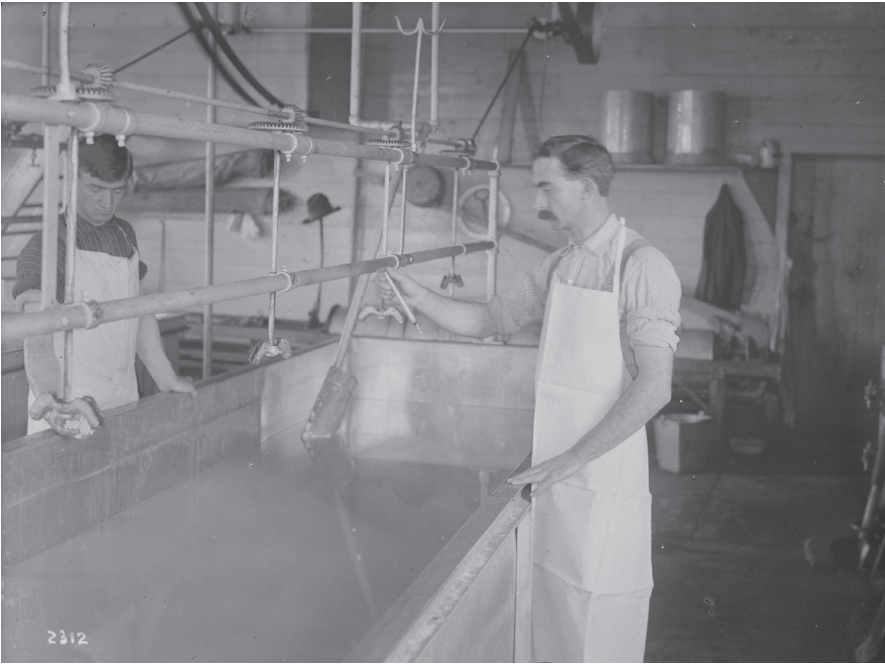
Figure 4. Taking temperature in cheese factory, n.d. The maker's use of a thermometer reflects the shift toward greater standardization of parts of the cheesemaking process while still depending on craft tools and methods.
